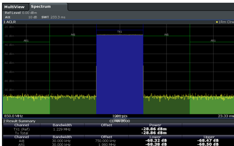
Figure 2-21: Measuring the channel power and adjacent channel power ratio for CDMA2000 signals with zero span (Fast ACLR)
