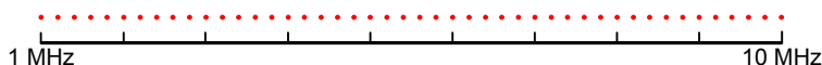
Figure 3-14: Linear x-axis scaling: the distance between the sweep points is equal, e.g. 200 kHz
